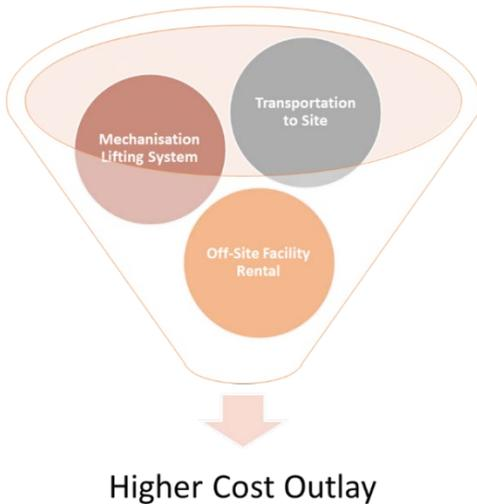
The estimated cost premium of adopting DfMA for MEP systems can range from approximately 10% to 30% of the total MEP construction cost depending on the type of building and MEP system, mainly driven by the requirements for off-site prefabrication facility and mechanism lifting system.
